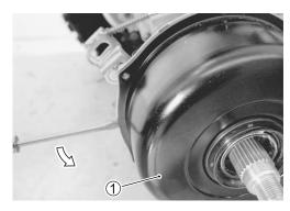
Remove the brake drum 2.
