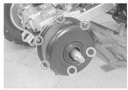
Remove the drum cover ① with a flat head screwdriver.
